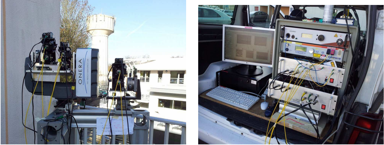
Figure 3. Lidar trial on water tower at ONERA Palaiseau (left) & Autonomous lidar operation from a car (right)
